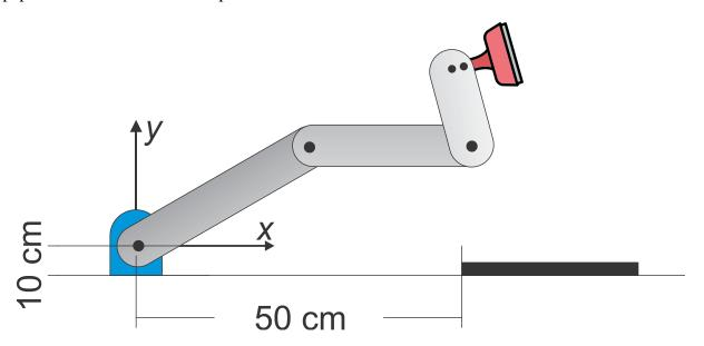
**Please calculate** valid workspace and joint positions for the final stamp location. **Then**, assuming initial arm angles of  $\theta_1=0^\circ$ ,  $\theta_2=15^\circ$ ,  $\theta_3=30^\circ$ , kindly calculate trajectory function so as to place the stamp correctly on the form regardless of where it is placed in the tray.
